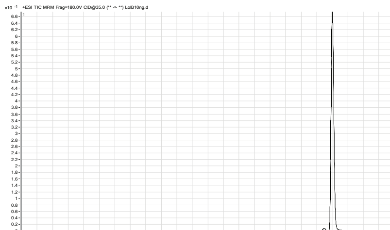
Figure 1. Total ion chromatogram of authentic standard of lolitrem B as separated via reversed-phase HPLC and detected via ESI LC-MS in multiple reaction mode (precursor ion=686 m/z, product ion=629 m/z). The small peak preceding the lolitrem B peak (the large peak at RT=10 min) is lolitrem F.
