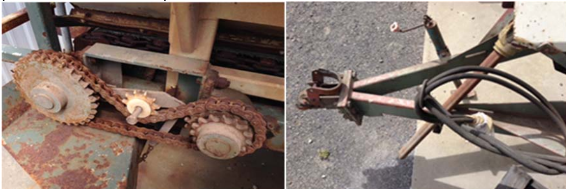
Chain guard missing
