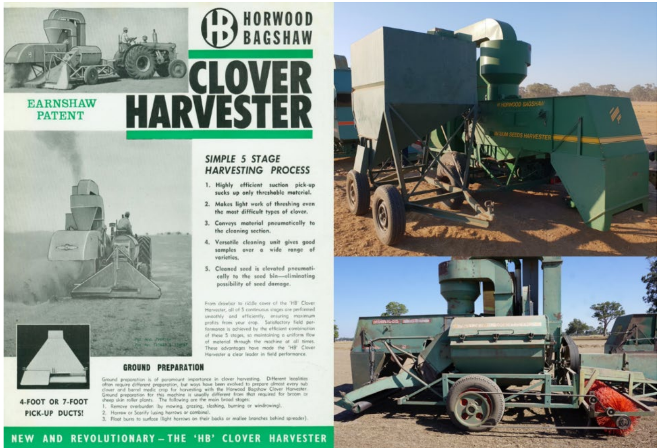
Figure 1. Left - Horwood Bagshaw Clover Harvester descriptive leaflet from 1964 (Horwood Bagshaw 1964). Top right – external seed bin addition. Bottom right – sweeper brush addition.
